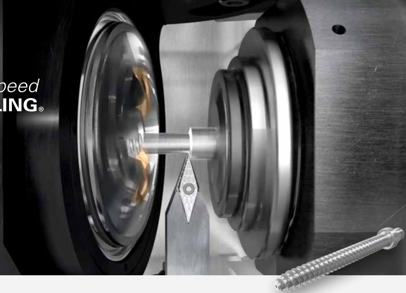
The high-speed whirling technique was developed for the production of bone screws with simultaneous turning and whirling operations. It offers considerable advantages for the manufacture of thread-type components, which are reflected in a reduction of production times, costs and an increased tool life.
